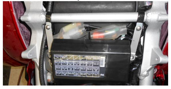
2. Secure with phillips screws, flat washers with nyloc nuts as shown.
