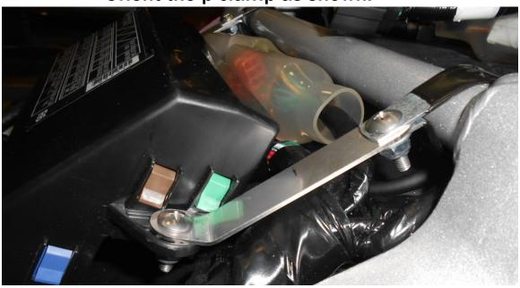
Orient the Relay Box as shown.
