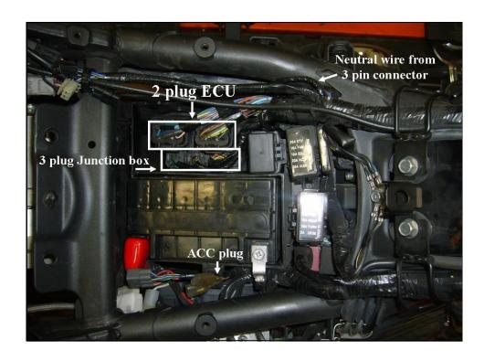
1. Locate the ECU (the 2 plug box) to the left of the battery.
