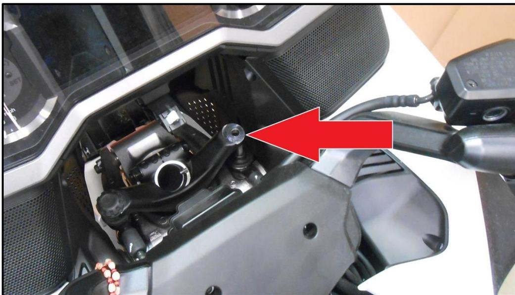
8. Remove the rubber cap on the right front Tie Rod nut and the plastic cap from the steering stem.
