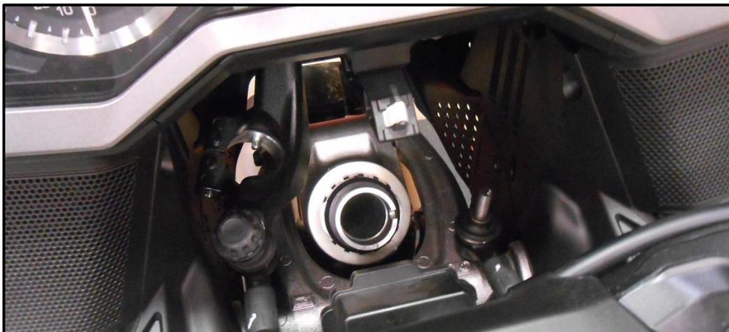
13. Remove the rubber seal and Lock washer.
