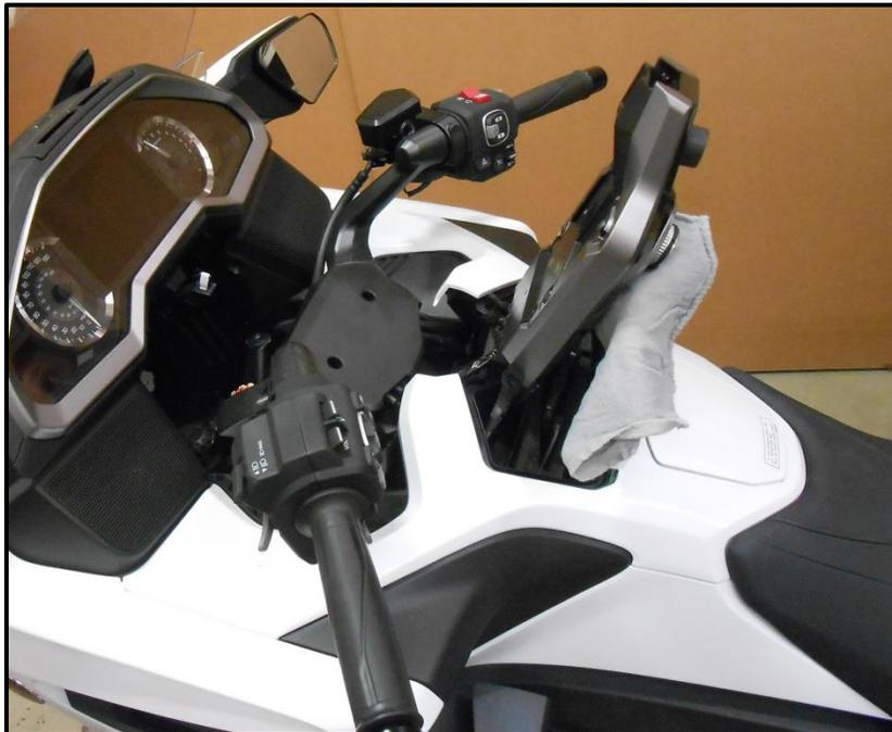
6. Remove 2 clips to pull up on the shelter, then remove 2 more push clips and 2 SHCS.
