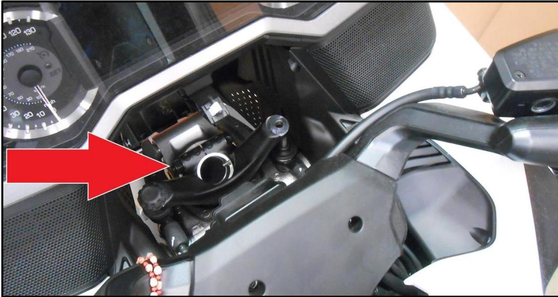
11. Remove the steering arm bolt and nut. **RED ARROW.**
